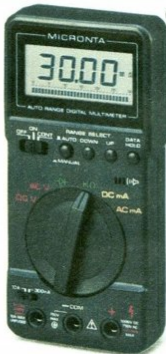
(5) Protective Holster, Autoranging/Manual, Bargraph. The 33-dot bargraph helps you spot peaks and trends. You also get a handy low-current range—200 μA! Data hold switch freezes display. Features include autopolarity, battery-saving automatic shutoff, continuity buzzer, and diode-check mode to test semiconductor junctions without damaging the devices. Measures to 1000 VDC, 700 VAC, 10 amps AC/DC current and 30 megohms resistance. 22-167 . . . 69.99
