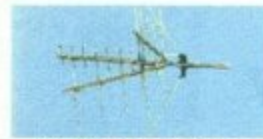
UHF yagi and corner reflector combination
